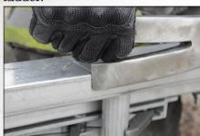
While holding the pike stationary, pull up on the fork end and rotate the forks over the beam.
