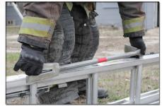
Arrange the bar so the pike is inside a rung with the bottom half of a fork overlapping the beam.
