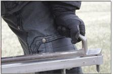
Secure the head of the roof hook inside the tip of the appropriate ladder.
